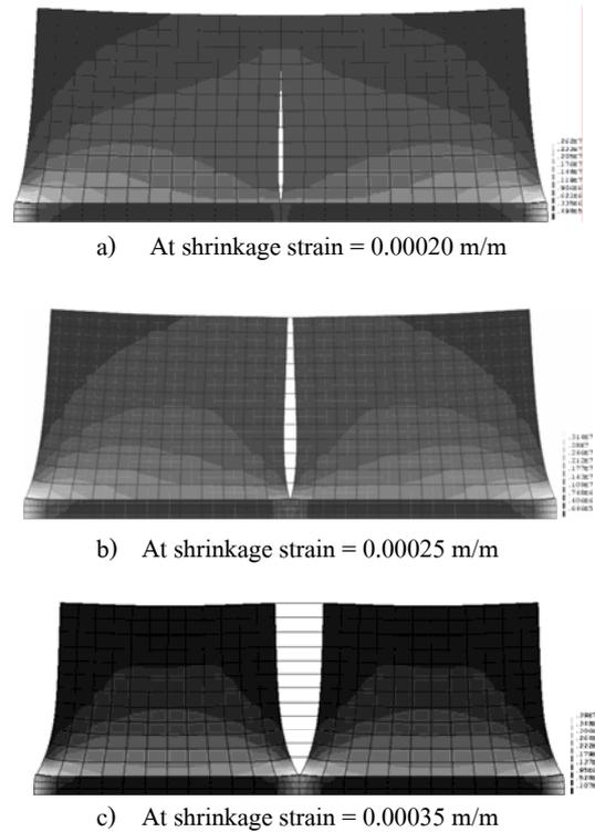
Figure 7. Progressive cracking in reference wall A
