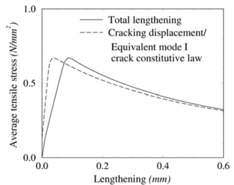
Figure 2. Wall part meso-analysis for the derivation of crack constitutive behaviour, to be employed as equivalent vertical crack constitutive law in macro-analysis [7]
