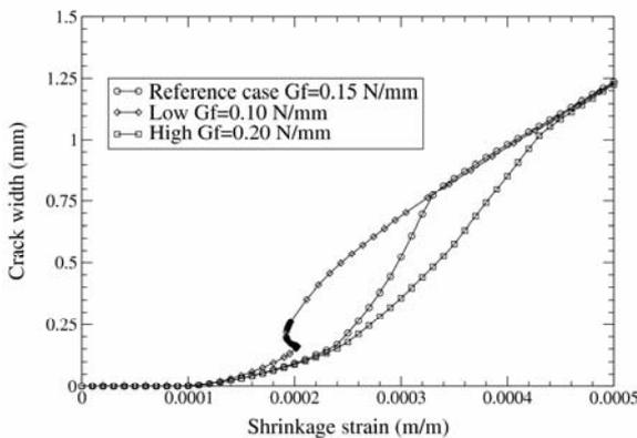
Figure 10. Influence of  $G_f$  on the shrinkage-crack width: walls A, D & E.
