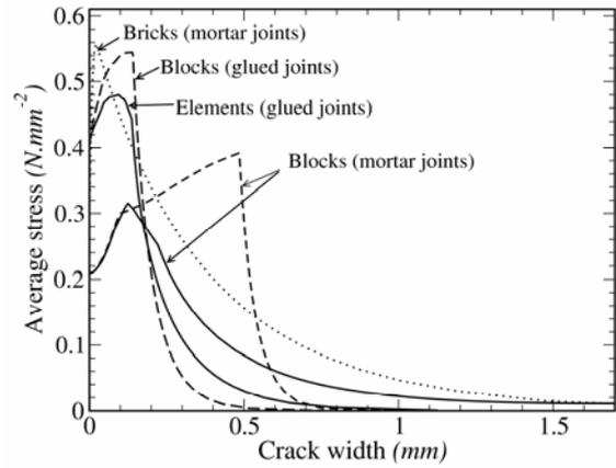
Figure 5. Constitutive behaviour for various calcium silicate masonry types, to be employed for the equivalent central crack in simplified restrained shrinking wall analyses.
