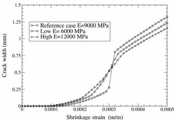
Figure 11. Influence of  $E$  on the shrinkage-crack width: walls A, F & G
