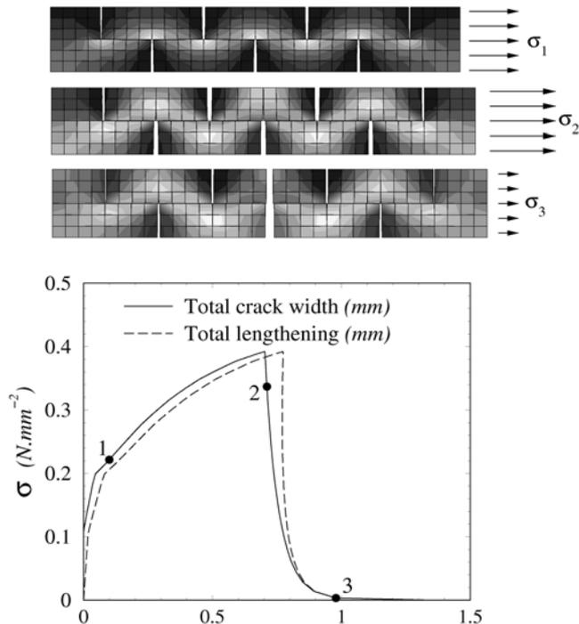
Figure 4. Typical derivation of the equivalent vertical crack constitutive behaviour.
