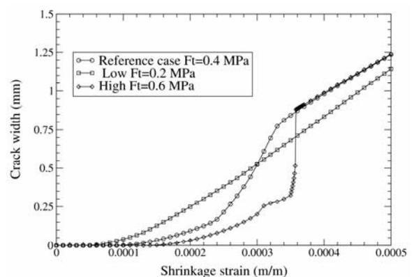
Figure 8. Influence of  $f_t$  on the shrinkage crack-width: walls A-C.
