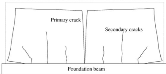
Figure 1. General crack pattern in base-restrained shrinking wall [7]
