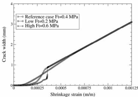
Figure 9. Influence of  $f_t$  on the shrinkage-crack width: Extended analysis
