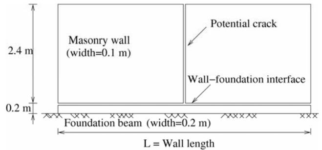
Figure 3. Simplified equivalent macro wall model
