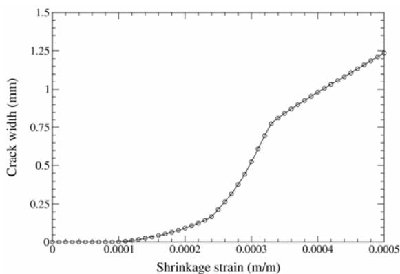
Figure 6. Shrinkage-crack width diagram of reference wall A
